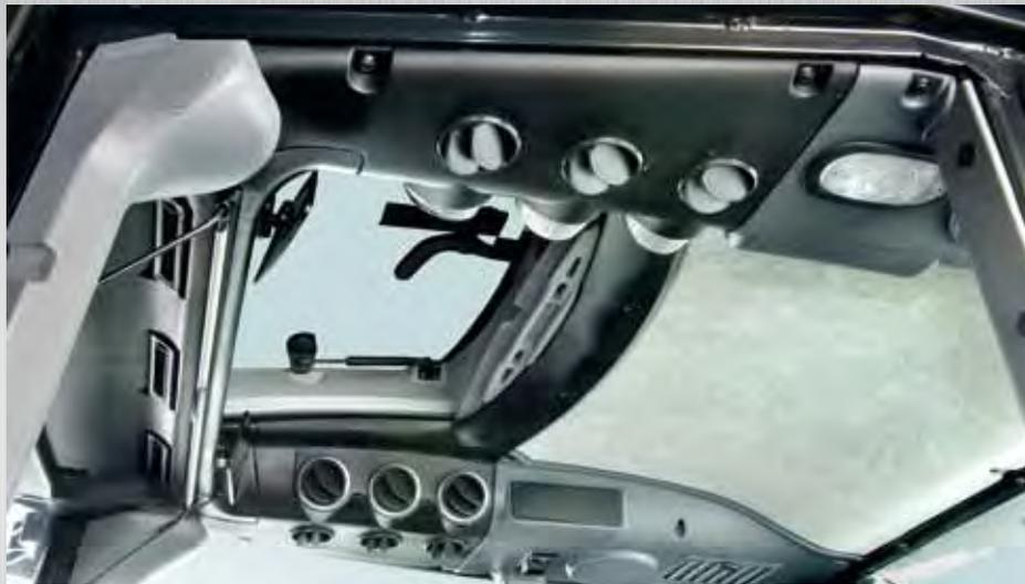
■ 4-speed ventilation system (air-conditioning optional) circulates a perfectly measured flow of air through 18 adjustable vents, regulating the temperature inside the cab at a level guaranteed to provide maximum operator comfort, whatever the climatic conditions.
