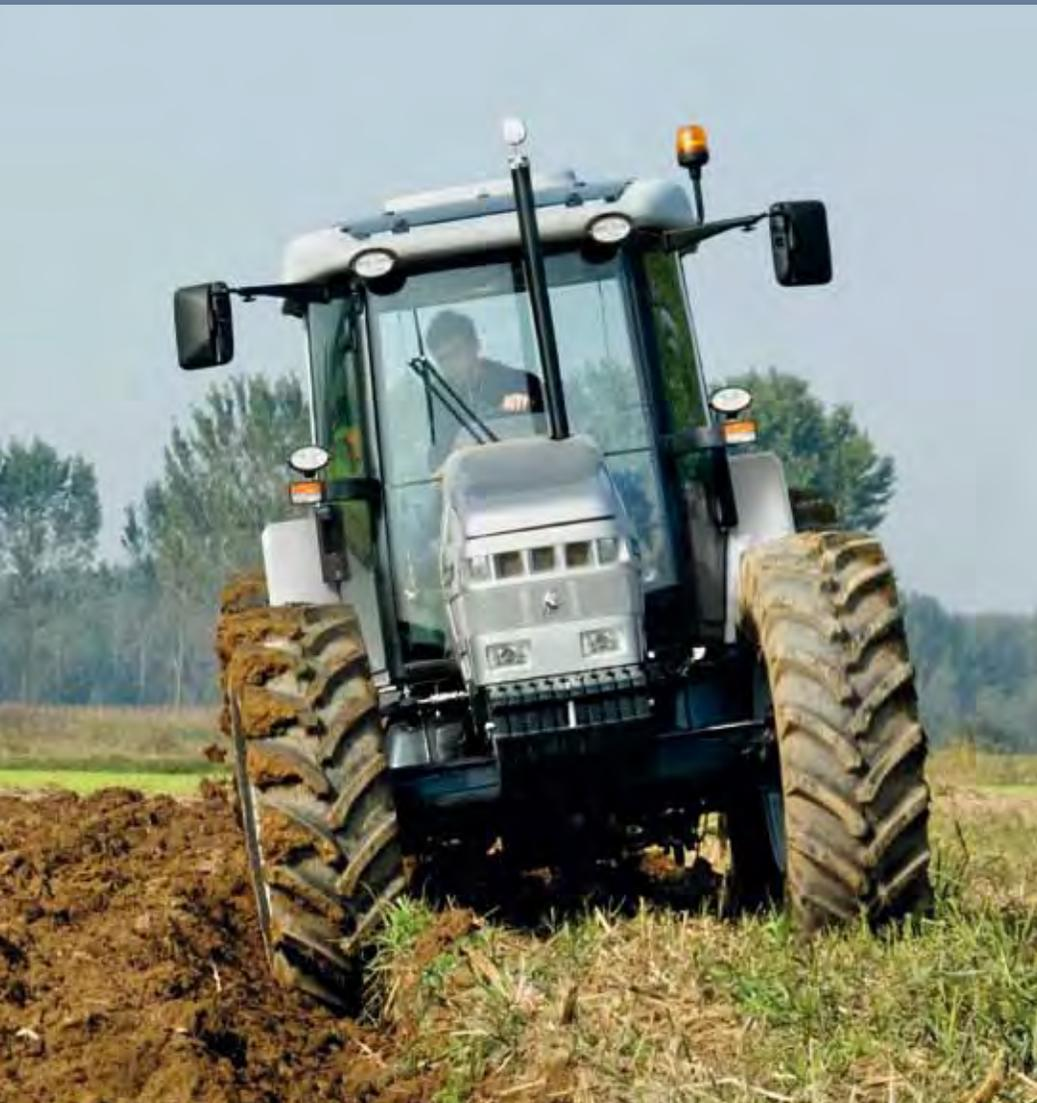
**An independent hydraulic circuit supplies oil for the power steering**, which is equipped with double cylinders giving a light and smooth touch at the wheel, and guarantees complete functional efficiency even at low engine speeds. The front axle features a 50° steering angle.
