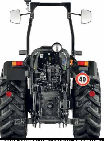
PRECISE CONTROL WITH MINIMAL EFFORT WITH A REAR LIFT HITCH CONTROL VALVE.
