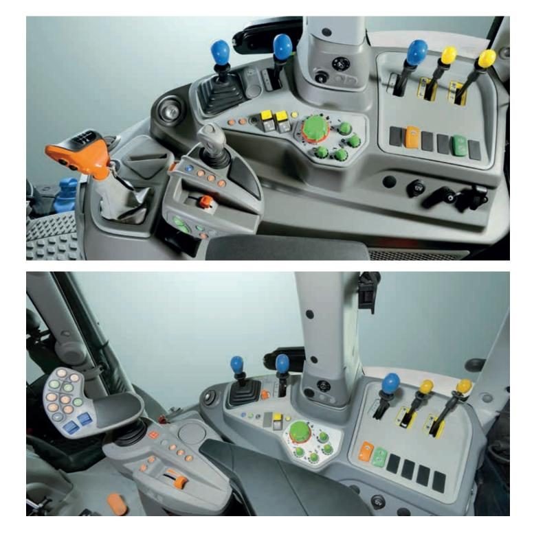
RCshift models are equipped with a completely automated transmission, with 5 robotically selected ranges managed entirely by exclusive software developed by Lamborghini Trattori, which, in addition to fully automatic mode, also offers the driver the choice of semi-automatic and manual modes.
