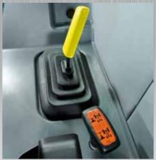
and fuel consumption reduced during operations with haymaking implements. The rear PTO is engaged mechanically by means of a lever on the left-hand side of the seat. A ground-speed PTO with independent output shaft is also available.
