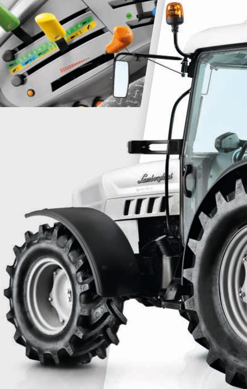
The best results from your lift, in all conditions. Draft and position control, mixed control mode and float mode are just some of the functions implemented automatically by the electronic lift, which uses a suite of integrated sensors to offer you total control in all situations.
