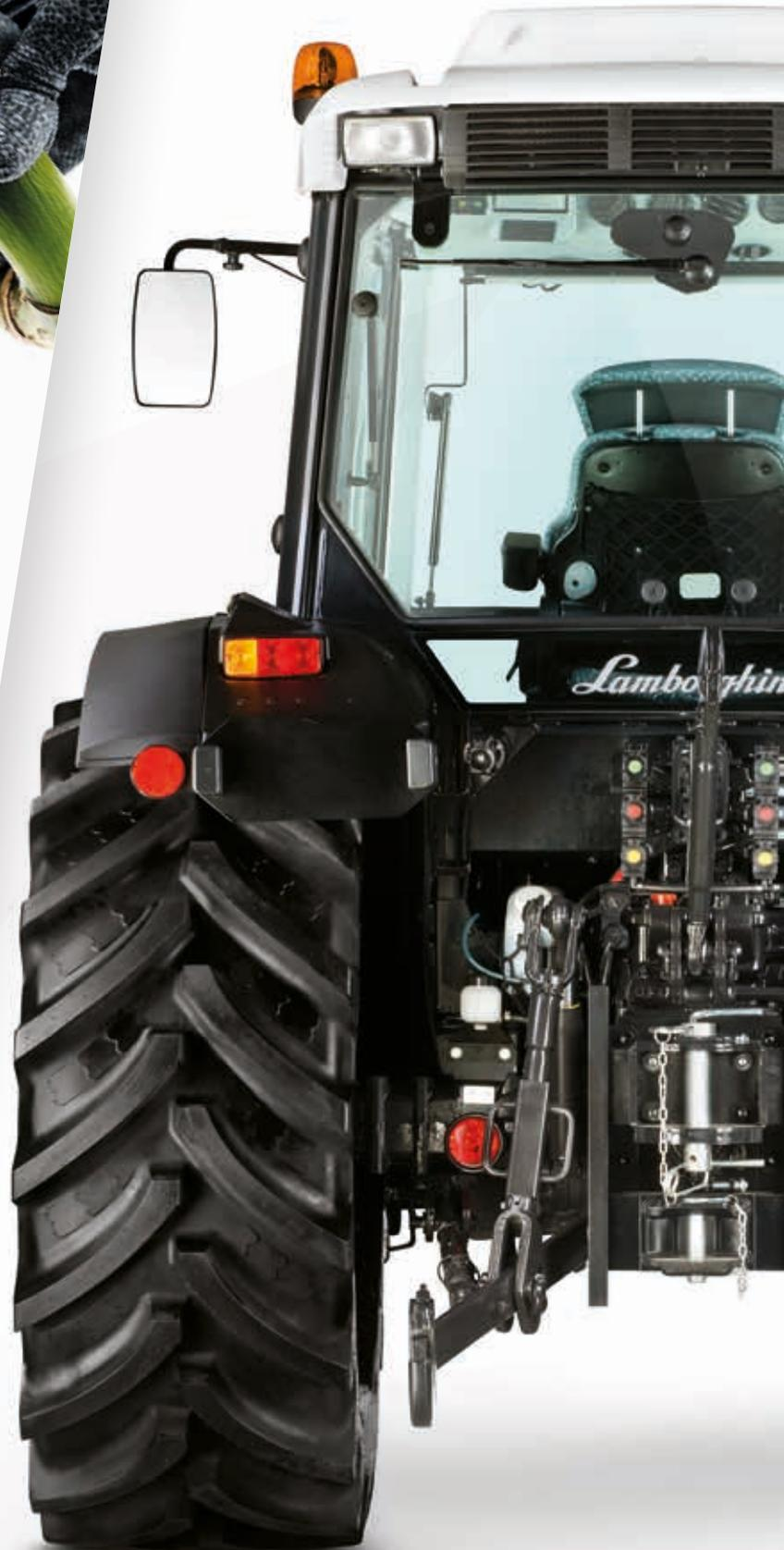
2-speed PTO (540/1000) – or with 540/540ECO/1000 speeds as an option – with multiplate wet clutch for Spire LS and GS tractors, or with a dry clutch for the Spire Target. A groundspeed PTO and a 1000 rpm front PTO are also available.
