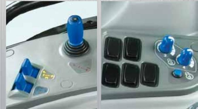
tuitive, using a practical cross-gate joystick (1<sup>st</sup> and 2<sup>nd</sup> spools) combined with fingertip levers (3<sup>rd</sup> and 4<sup>th</sup> spools).
