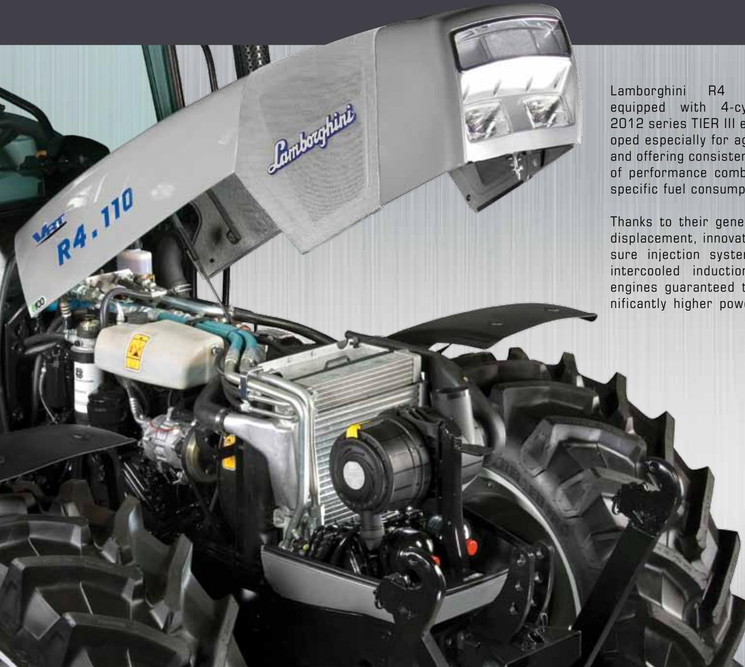
Lamborghini R4 models are equipped with 4-cylinder Deutz 2012 series TIER III engines, developed especially for agricultural use and offering consistently high levels of performance combined with low specific fuel consumption.
