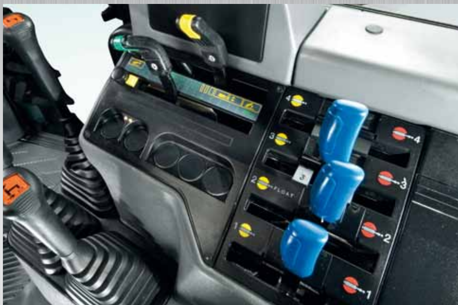
■ Two levers are used to control the rear lift links: the yellow lever raises or lowers the implement; the green lever is used to select the type of control (position, draft, mix and float). The blue levers operate the various auxiliary spools - single acting, double acting, kickout or detent.
