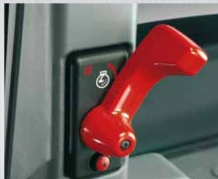
■ Control lever on the cab door pillar, allowing variation of engine speed. Function for setting a preferred engine speed.
