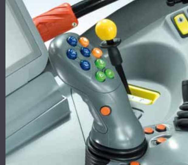
■ PowerComS joystick - all functions within easy reach: hydraulic system, transmission and rear lift.
