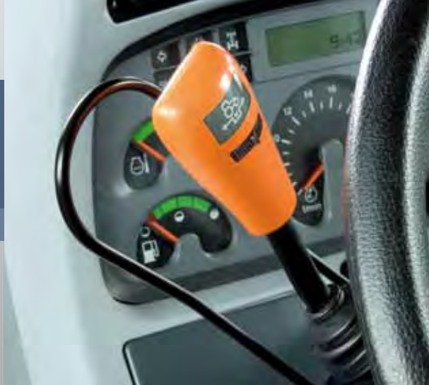
■ The shuttle lever is located beneath the steering wheel. Ergonomically designed and easy to use, it has a "neutral" position and will function only when enabled, to ensure total safety in operation.
