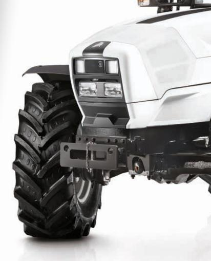
$55^\circ$  for 4 wheel drive versions and 70° for 2 wheel drive versions: the steering angle of the Spire lets you work effectively even in the tightest situations.
