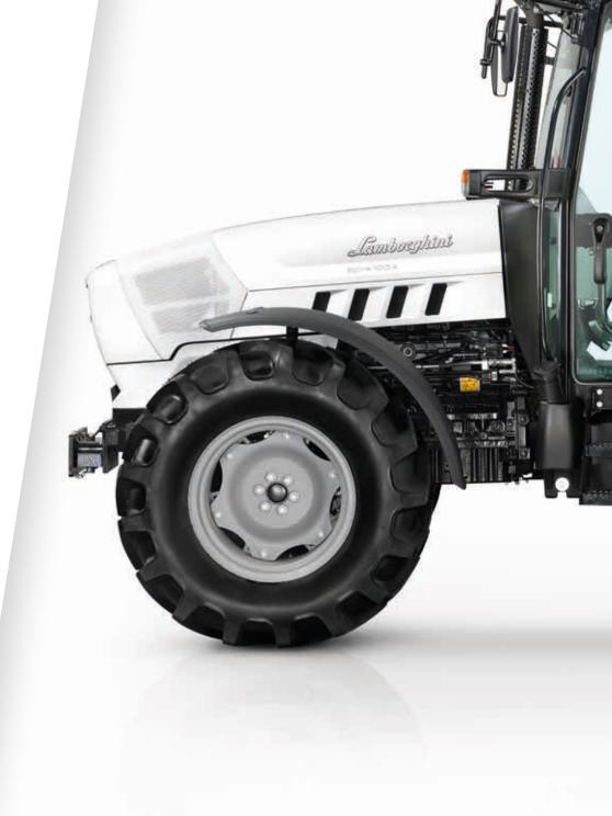
The hydraulic power shuttle with SenseClutch saves time when inverting direction and performing headland turns. The two Long Life multiplate wet clutches and electronic control unit work in conjunction to reduce strain and wear and keep the mechanical components of the system in perfect working order.
