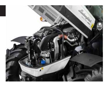
catalytic converter is positioned in a sheltered, protected area along with the new PowerCore 2-stage air filter (which can be fitted upon request with a dust ejector). To facilitate maintenance, all inspection and service points have been made more easy to access, and the radiator pack is now protected by two practical sliding screens.
