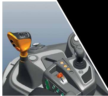
range gearbox, for a total of 30+15 speeds (which may be increased to 54+27 speeds with the addition of underdrive). All transmission variants feature a hydraulic reverse shuttle, the button-operated ComfortClutch system (for shifting without using the clutch pedal), and the Stop&Go and SpeedMatching functions. The use of proportional selector valves offers a smooth shift action comparable to a VRT transmission but with the typical efficiency of a mechanical Powershift range gearbox.
