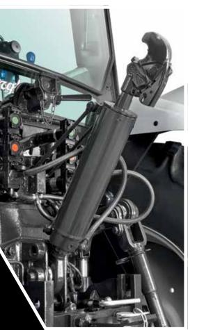
lift and a 1000 rpm front PTO - the ideal solution for tasks requiring simultaneous use of front and rear implement and for hitching ballast. The capabilities of the hydraulic system may be extended even further with an innovative 60ECO dual pump, which already delivers a flow rate of 60 I/min at an engine speed of just 1600 rpm.
