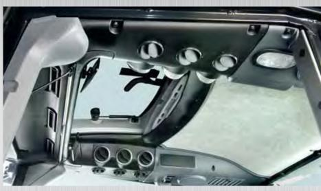
4-speed ventilation system (air-conditioning optional) circulates a perfectly measured flow of air through 18 adjustable vents, regulating the temperature inside the cab at a level guaranteed to provide maximum operator comfort, whatever the climatic conditions.
