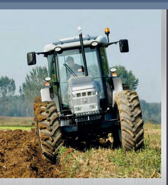
An independent hydraulic circuit supplies oil for the power steering, which is equipped with double cylinders giving a light and smooth touch at the wheel, and guarantees complete functional efficiency even at low engine speeds The front axle features a 50° steering angle.
