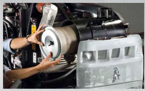
Simplified routine maintenance checks. The hood opens simply by pushing a button on the front panel. The side panels are removable without any need for tools.
